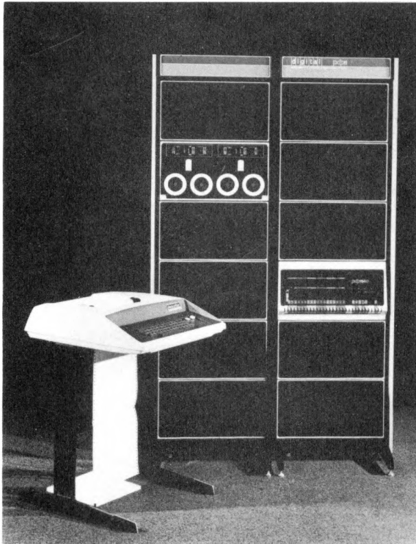
A dual cabinet version of Digital Equipment's PDP-11/40 computer. One of Digital's famous PDP-11 family of 16-bit computers.
